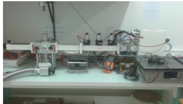
2.45GHz Single mode resonant-cavity
