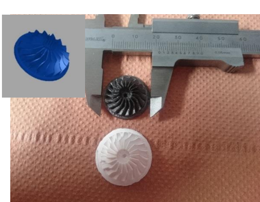
Turbine – Tool 40mm 1600°C-10min-3kN
